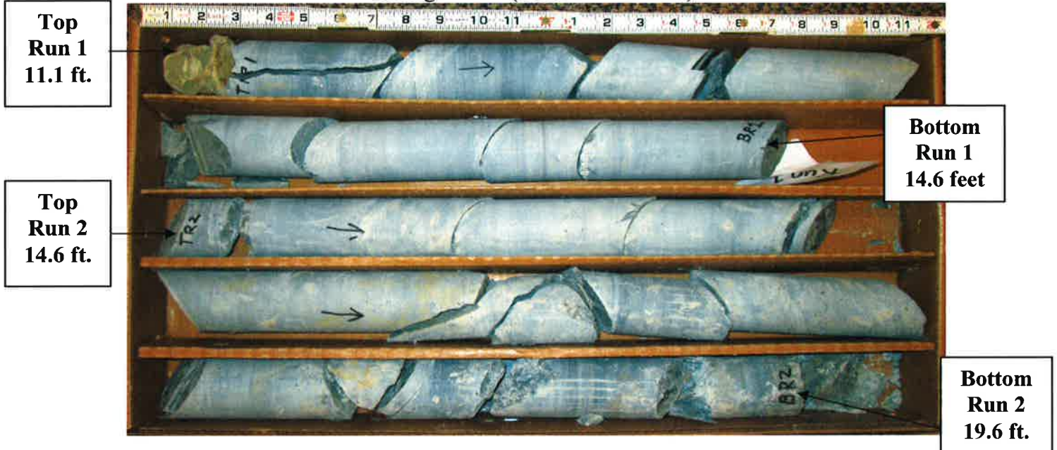
Boring EB1-B (Core Run 3)
